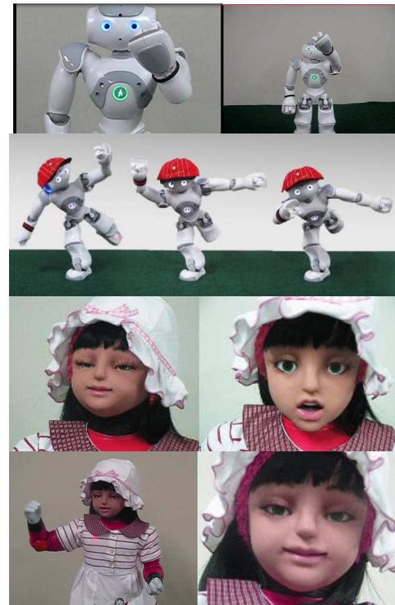
Fig. 6. NAO and Alice robots in autism treatment process (teaching colors, pointing to a picture, one-leg balance, waving, and smiling)
