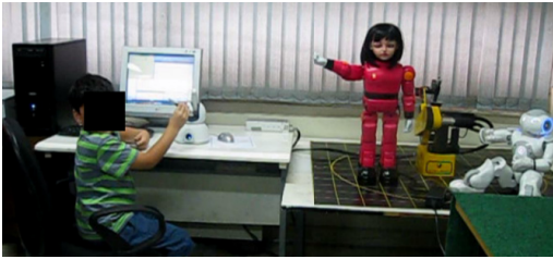
Fig. 3. Teleoperating Robots using the Haptic Phantom Omni robot- Game#3.
